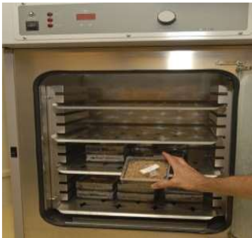
Figure 3. The accelerated aging technique of the seed vigor test
